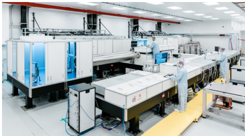
L4 laser system at ELI Beamlines (10 PW, 1.5 kJ, 150 fs, 1057 nm)
