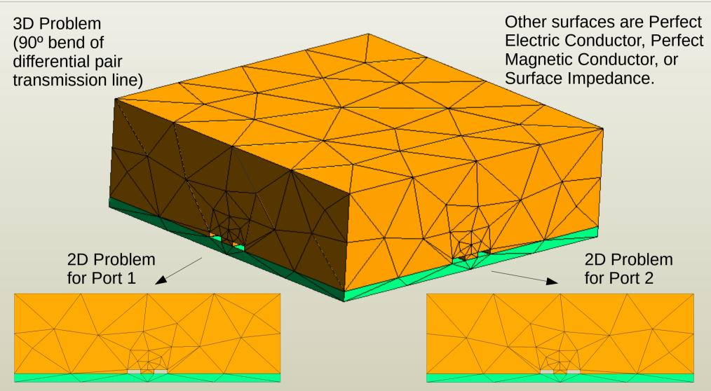
2D solutions solve for the EM fields, propagation constants, and characteristic impedances.
