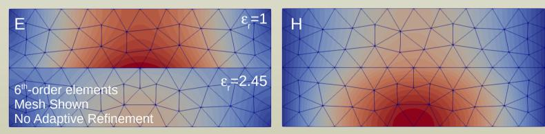
**Partially-Filled Rectangular Waveguide**
